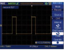
Monitor and analyze long-term signal behavior by recording data continuously over an extensive period of time and playing them back for post acquisition analysis. Data is recorded in a sequence of up to 2500 frames.
