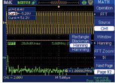
Display and measure the input signal's frequency spectrum. Select one of the 4 FFT windows: Rectangular, Hanning, Hamming, and Blackman. Use cursors to measure the spectral component's magnitude and frequency.
