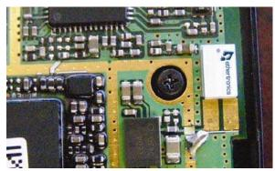
Ethertronics' Savvi series of Isolated Magnetic Dipole<sup>™</sup>(IMD) antennas deliver on the key needs of device designers for higher functionality and performance in smaller/thinner designs. These innovative antennas provide compelling advantages for ISM enabled M2M, tracking and smart metering applications.
