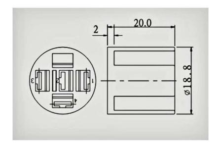
MATERIAL: Frames are nylon (UL Flame: 94V-2).
