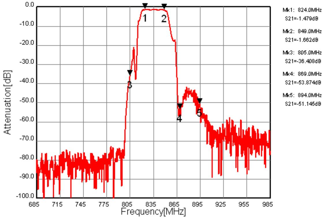
Fig.1 Pass-band Characteristics
