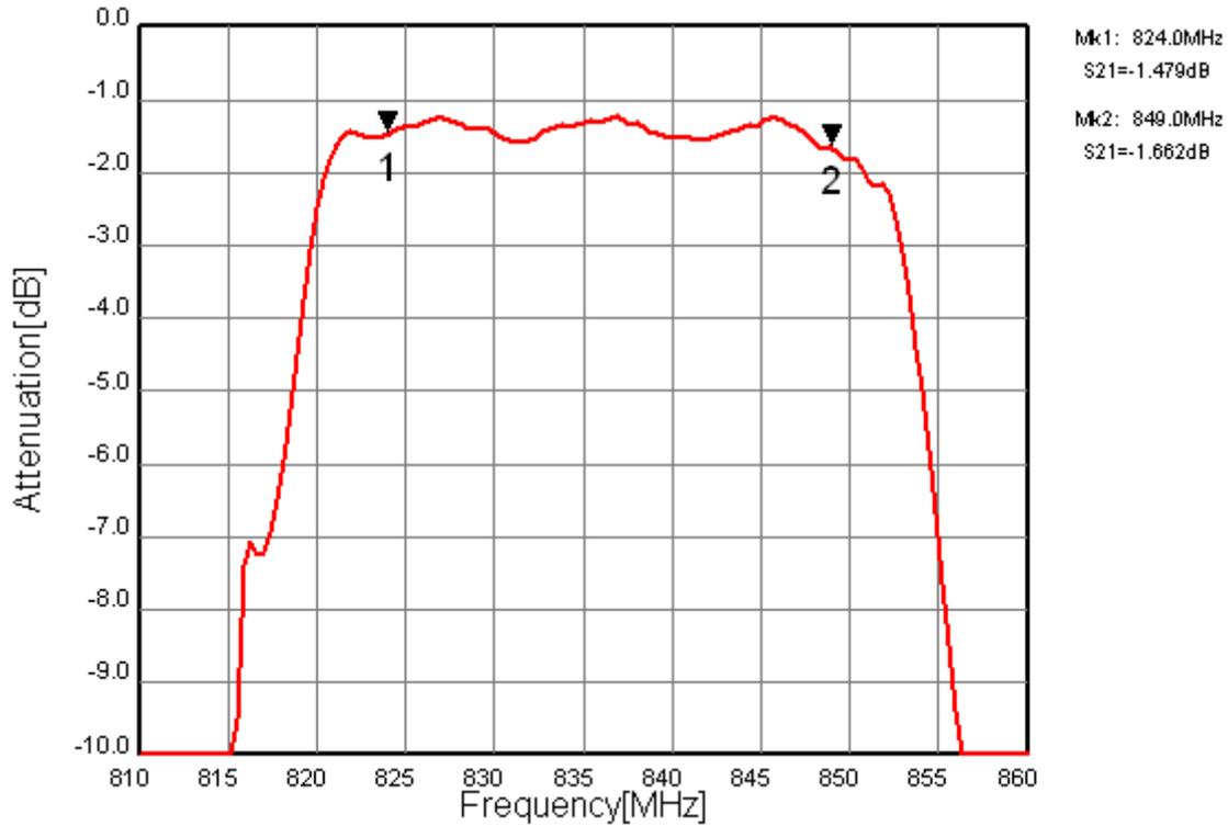
Fig.3 In-band Characteristics
