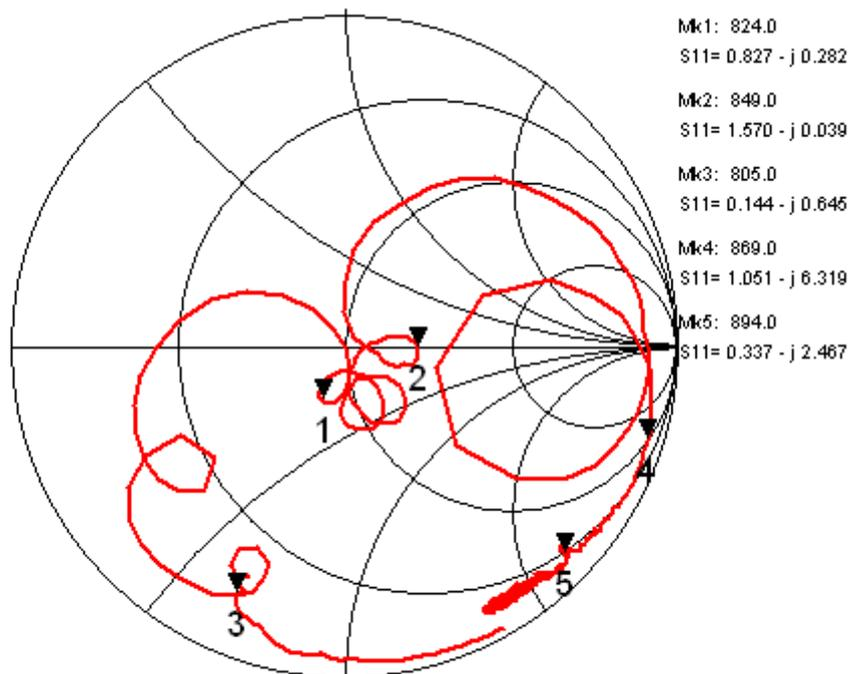
Fig.6 Output Impedance (Unbalance)
