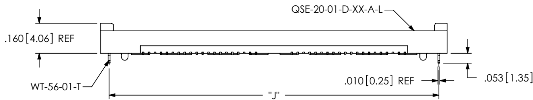
FIG 8 -L: LATCHING OPTION (QSE-020-01-XXX-D-DP-A-L SHOWN) (DIFFERENT AS SHOWN, OTHERWISE SAME AS FIG 1) (MUST USE -A OPTION) (MAXIMUM 28 POS) (NOT AVAILABLE WITH -LC, -GP, -FL, OR -RT1)
