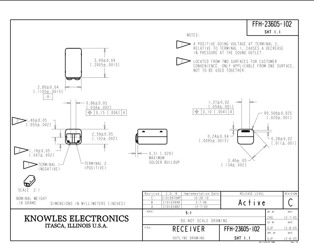
THE FFH-23605-102 IS A FERROFLUID DAMPED FH-23605 RECEIVER WITH A PEAK OF 2dB RELATIVE TO THE SENSITIVITY AT IKHZ UNDER CONSTANT VOLTAGE DRIVE CONDITIONS.
