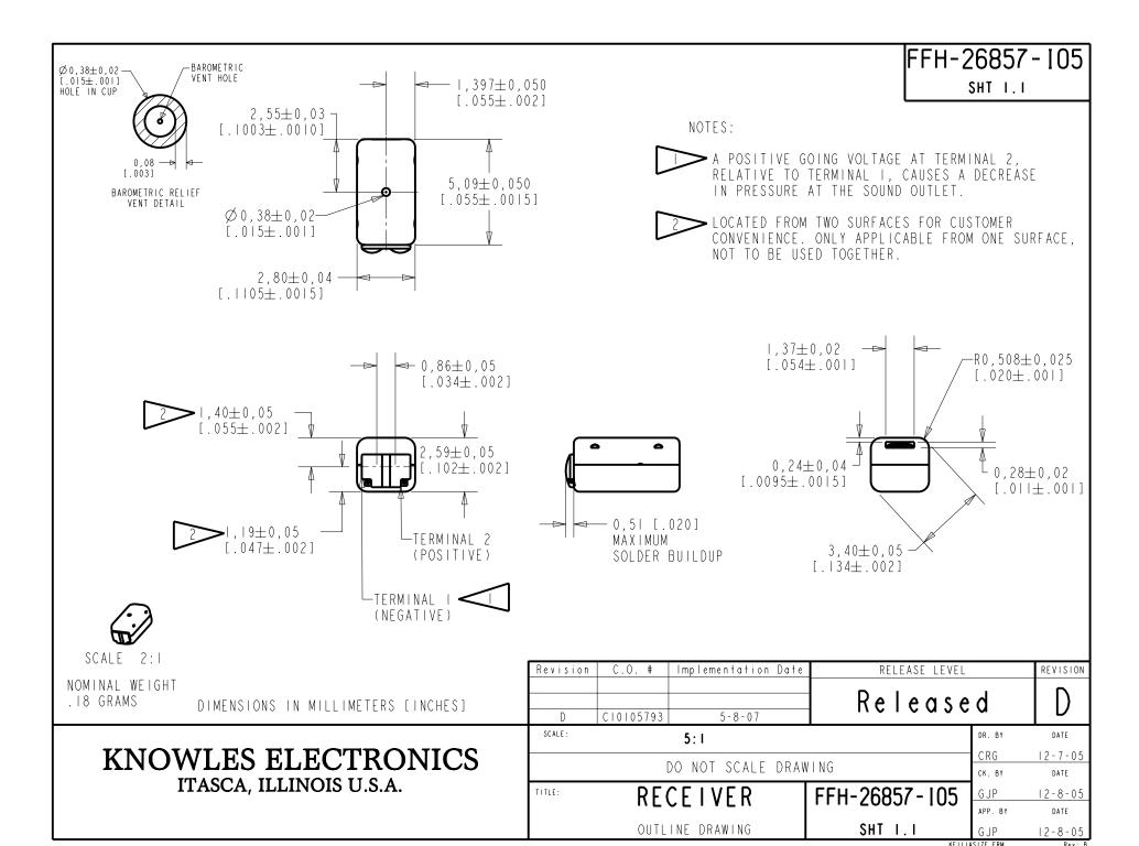
THE FFH-26857-105 IS A FERROFLUID DAMPED AND EXTERNALLY VENTED FH-6553 RECEIVER WITH A PEAK OF 5dB RELATIVE TO THE SENSITIVITY
