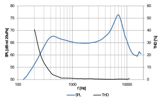
measured in IEC baffle with open back volume (10mW, 10cm)
