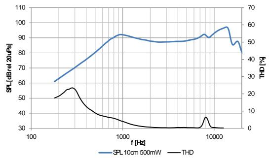
measured in IEC Baffle at 500mW in 10cm distance with 1 ccm back cavity
