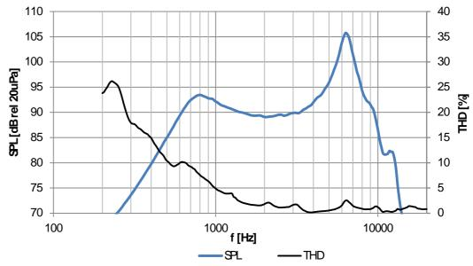
measured in IEC baffle at 420mW in 10 cm distance with 1ccm back cavity
