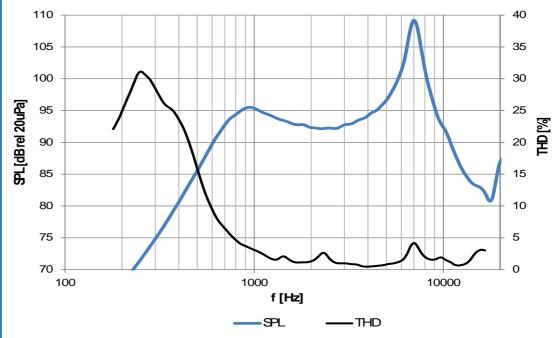
measured in IEC baffle at 1000mW in 10 cm distance with 1ccm back cavity
