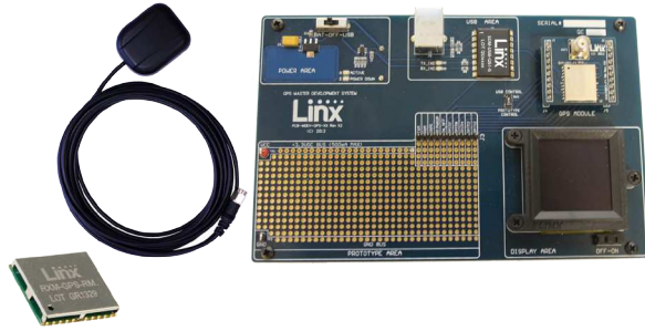
Figure 36: The RM Series Master Development System
