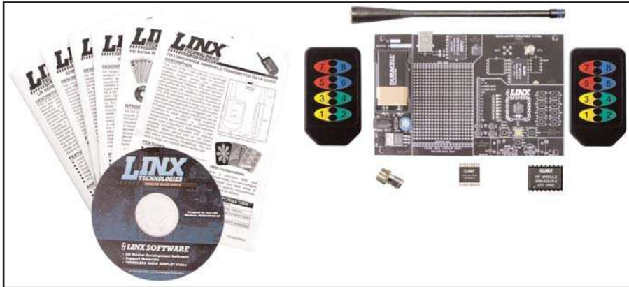
Figure 8: OTX-***-HH-CP8-HS Master Development System
