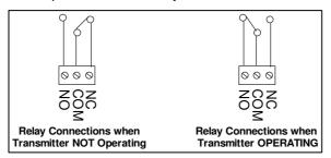
Relay output '1' provides a longer momentary output (approx ½ second) this may be removed (see below). For solenoid driven traps.
