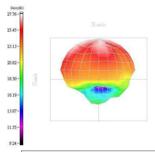
Max gain= 27.76dBi, at (0, 195) Average Power= 19.78dBm Directivity(dB)= 4.48 Efficiency= 19.28dB, 8462.62%
