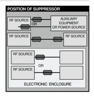
**POSITION OF SUPPRESSOR** The suppressor should normally be located close to the cable termination where it exits the enclosure. Where a cable connects two enclosures containing RF sources, a suppressor on each end may be required. For circuits within an enclosure, a position close to the RF is best. However, other locations along the circuit may work as well.
