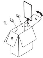
Insert handles before folding up box. Place shorter dimension of wire on crease where flap A & box meet.
