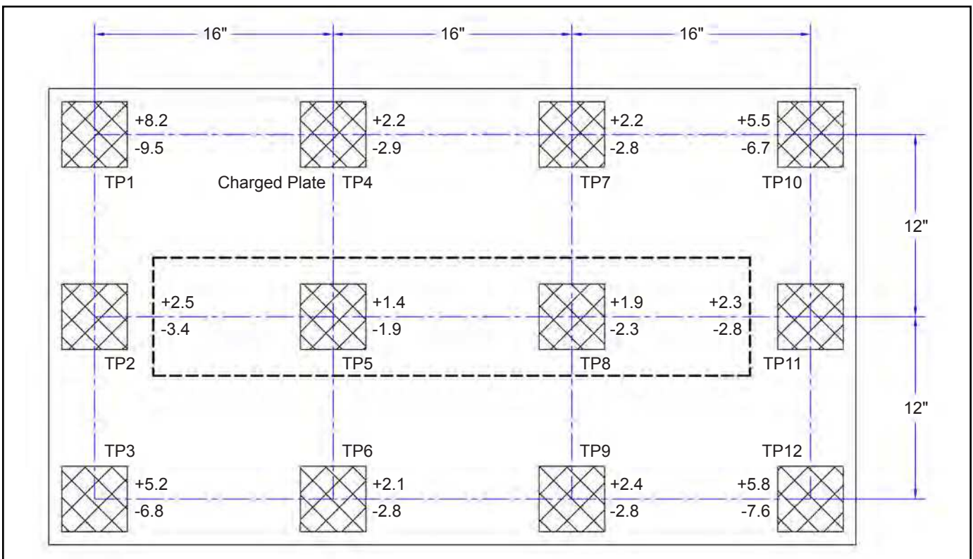
Figure 8. 60473 Neutralization (Discharge) Times at 120VAC, 60Hz input
