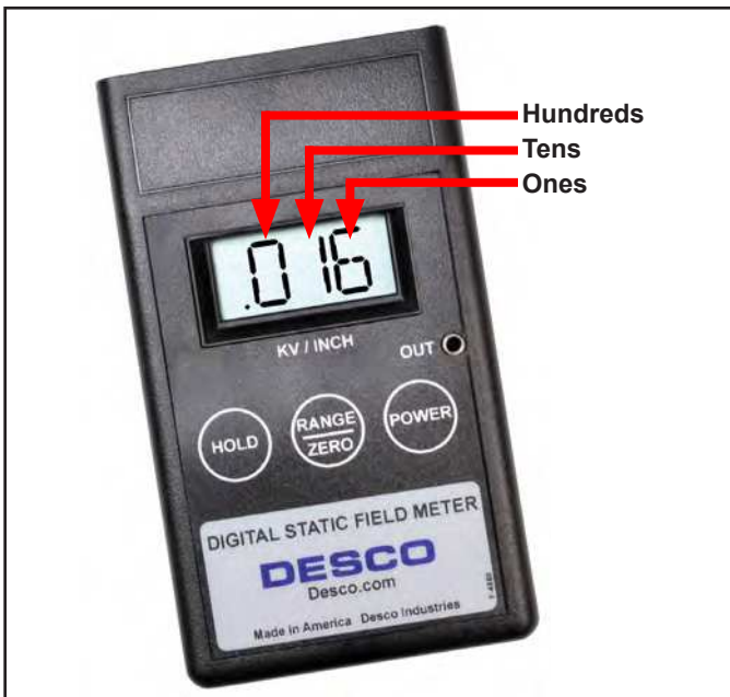
Figure 4. Reading the Digital Static Field Meter while in the \pm 2 kV range
