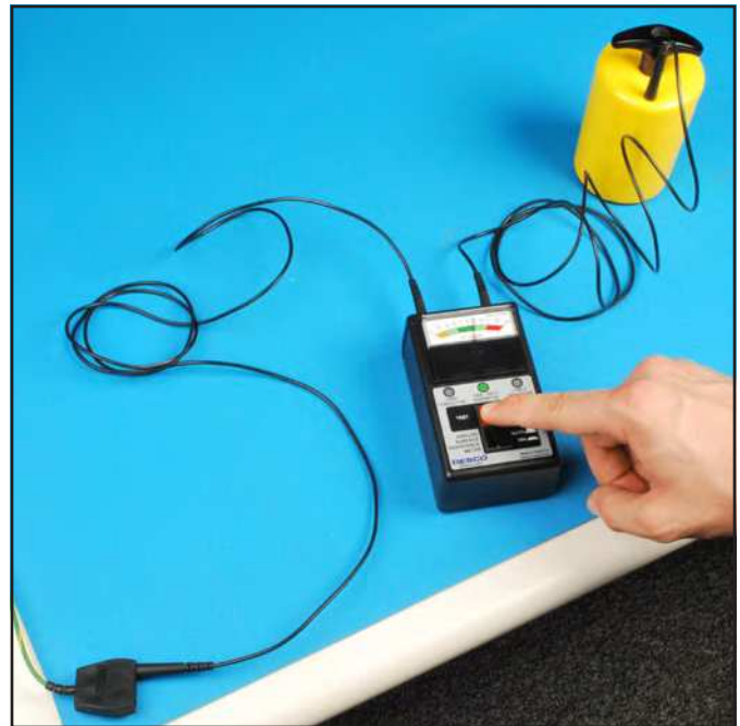
Figure 3. Using the test leads and one 5 pound electrode to measure RTG
