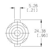
SPECIFICATION: BODY: HIGH IMPACT ABS, UL94V-HB, FILE NO. E56070(S)
