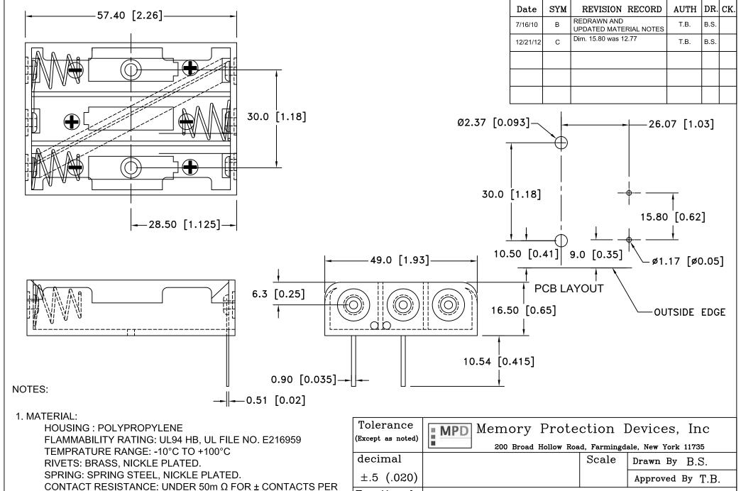
EIA-540J000 ROHS COMPLIANT (Except as noted) 200 Broad Hollow Road, Farmingdale, New York 11735 decimal  $\pm .5 \text{ (.020)}$  Scale Drawn By B.S. Approved By T.B. Fractional  $\pm .8 \text{ (.030)}$  Title THREE "AA" CELL HOLDER  $\pm .8 \text{ (.030)}$  Date Drawing Number  $\pm .3^{\circ}$  12/21/12 BC3AAPC
