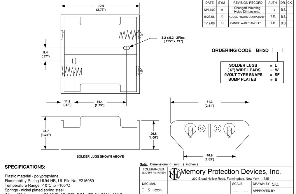
Wire - 152.4 mm Long 26 AWG, UL1007, CSA - TR-64, 300V, 80°C. Rivets - Brass, nickel plated 9 Volts Snaps - Brass, nickel plated Contact Resistance: Under 50 Ω for +/- contacts per EIA-540J000 ROHS COMPLIANT
