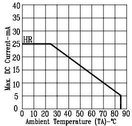
Fig5. MAX. ALLOWABLE DC CURRENT VS. AMBIENT TEMPERATURE.
