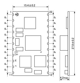
Tolerance is not accumulated. 【Unit:mm】 Marking (1) Pin No.1 Marking / MFG ID (M PMF: MPDTY301S (2)Parts No. PMK: MPDTY302S (3) Lot No  $\Box\Box$ (1)(2)(1)Production Year 2 Production Month (1,2,3,…9,O,N,D)
