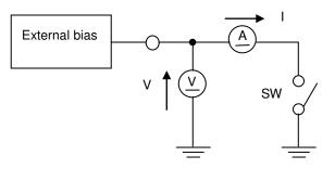
External bias voltage shall be measured when SW left open. External bias current shall be measured when SW left short.
