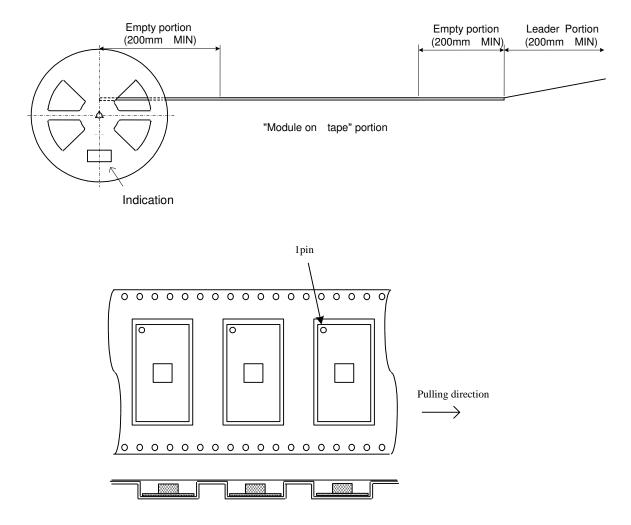
The module is located such as parts in upper side and PCB in lower side.
