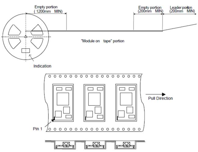
The module is oriented such that the inductor coil is located on the top side and the terminal pins on the bottom side
