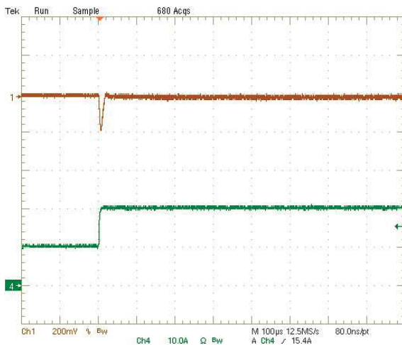
Step Load Transient Response (Vin=5.0V, Vout=2.5V, Cload=94µF, Iout=6A to 12A) Trace 1=Vout, 200 mV/div, Trace 4=Iout, 10A/div.
