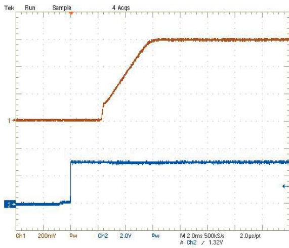
Step Load Transient Response (Vin=5V, Vout=0.6V, Cload=94µF, Iout=6A to 12A) Trace 1=Vout, 200 mV/div, Trace 4=Iout, 10A/div.
