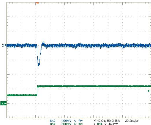
Step Load Transient Response (Vin=12V, Vout=1.2V, Clod=0, Iout=1.5A to 3A) Trace 2=Vout, 100 mV/div. Trace 4=Iout, 2.5A/div.
