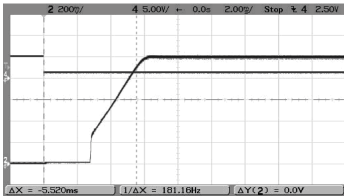
On/Off Enable Delay (Vin=12V, Vout=1.0V, Iout=6A, Load=0) Trace 4=Enable, Trace 2=Vout
