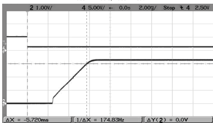
On/Off Enable Delay (Vin=12V, Vout=3.3V, Iout=6A, Load=0) Trace 4=Enable, Trace 2=Vout
