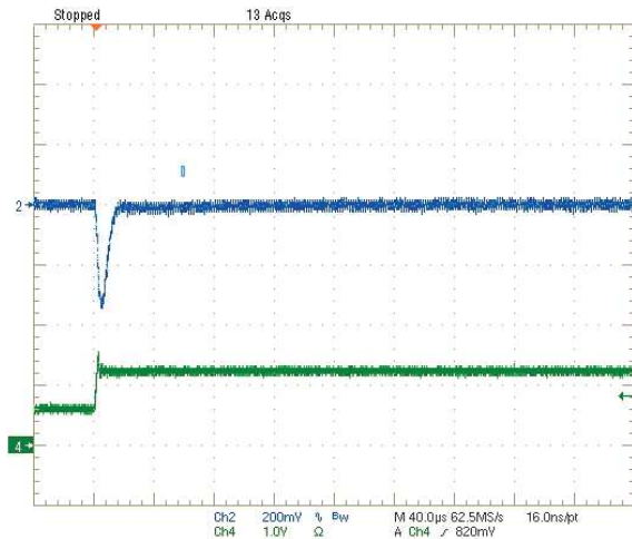
Step Load Transient Response (Vin=12V, Vout=1.8V, Load=0, Iout=3A to 6A) Trace 2=Vout, 200 mV/div. Trace 4=Iout, 5A/div.
