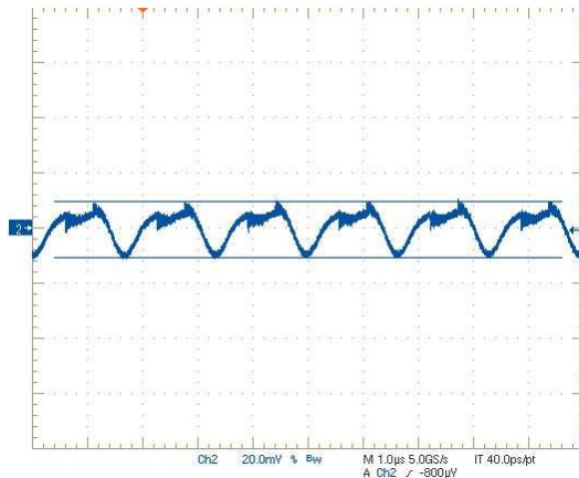
Step Load Transient Response (V in =5V, V out =3.3V, I out =6A to 3A) Trace 2=V out , 200 mV/div. Trace 4=I out , 5A/div.
