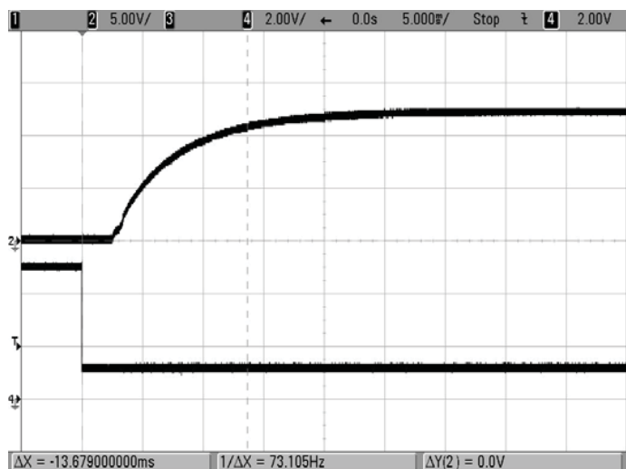
Enable Start-up (Vin=48V, Iout=5A, Cload=1000uF Ta=+25°C) Trace 2=Output, Trace 4= Enable.
