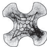
4-Indenter Crimp Cross-section Across Axis
