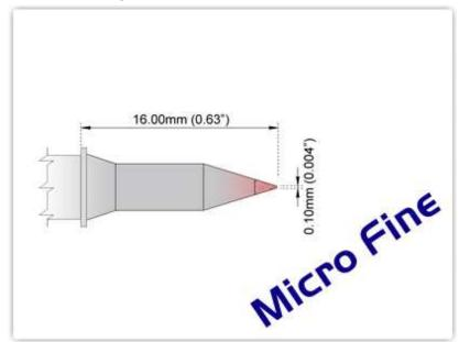
EBM7 C001 Conical 0.10mm (0.004"), Micro Fine
