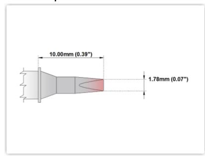
EBM7CH176 Chisel, 1.78mm (0.07"), 30°
