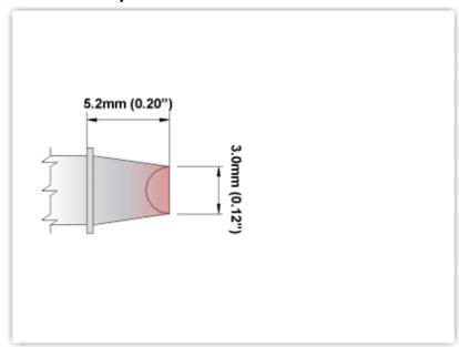
EBM7CH181 Chisel, 3.00mm (0.12"), 90°
