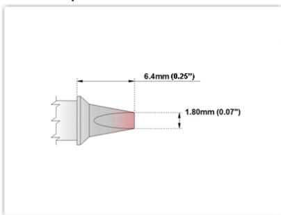
EBM7CP201 Chisel, 1.80mm (0.07"), 30°
