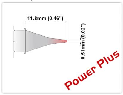
EBM7CS152H Conical Sharp 0.5mm (0.02"), Power Plus
