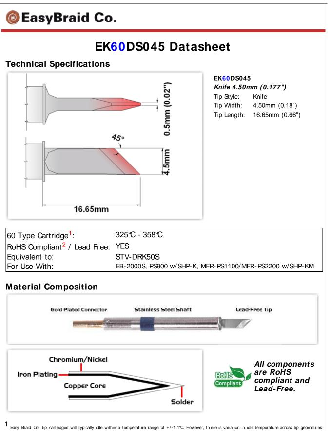
Leasy Braid Co. tip cartridges will typically idle within a temperature range of +/-1.1°C. However, there is variation in idle temperature across tip geometries within an individual temperature series. Easy Braid Co. offers a wide variety of tip geometries from 0.25mm fine point tip to 5mm chisel. The length and geometry of a tip will have an influence on the tip idle temperature. To accurately measure idle temperature it will depend greatly on the measurement method,
