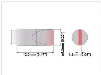
EP75 CH052 Chisel 30° 5.20mm (0.20")
