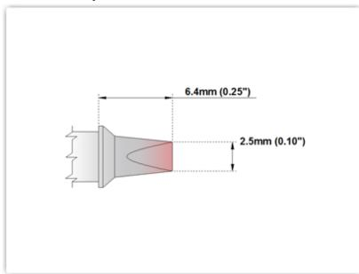
EPM75CP200 Chisel 30° 2.5mm (0.10") Tip Style: Chisel 30°
