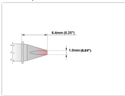
ETM70CH179 Chisel 30° 1.0mm (0.04")
