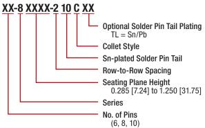
ALL DIMENSIONS: INCHES [MILLIMETERS] ALL TOLERANCES: ±0.005 [0.13] UNLESS OTHERWISE SPECIFIED FOR COLLET CONTACTS ON 0.300 [7.62] CENTERS, SEE DATA SHEET 13008 FOR BIFURCATED CONTACTS, SEE DATA SHEET 13006 CONSULT FACTORY FOR OTHER SIZES AND CONFIGURATIONS
