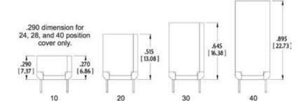
ALL DIMENSIONS: INCHES [MILLIMETERS] ALL TOLERANCES: ±0.005 [0.13] UNLESS OTHERWISE SPECIFIED FOR MATING DIP HEADER, SEE <u>DATA SHEET 12032</u> CONSULT FACTORY FOR OTHER SIZES AND CONFIGURATIONS CUSTOMIZATION: ARIES SPECIALIZES IN CUSTOM DESIGN AND PRODUCTION. SPECIAL MATERIALS, PLATINGS, SIZES, AND CONFIGURATIONS CAN BE FURNISHED, DEPENDING ON QUANTITY.
