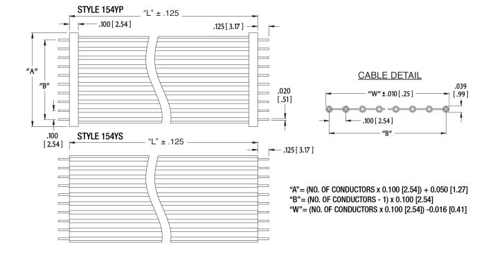
ALL DIMENSIONS: INCHES [MILLIMETERS] ALL TOLERANCES: ±0.005 [0.13] UNLESS OTHERWISE SPECIFIED NOT TO BE USED FOR HIGH-FLEX APPLICATIONS FOR HIGH-FLEX APPLICATIONS, SEE <u>DATA SHEETS 11005</u> & <u>11014</u> CONSULT FACTORY FOR OTHER SIZES AND CONFIGURATIONS CUSTOMIZATION: ARIES SPECIALIZES IN CUSTOM DESIGN AND PRODUCTION. SPECIAL MATERIALS, PLATINGS, SIZES, AND CONFIGURATIONS CAN BE FURNISHED, DEPENDING ON QUANTITY.
