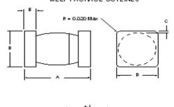
Note: Cathode side of device is indicated by a dark band marked on body.
