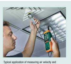
Typical application of measuring air velocity and temperature in HVAC
