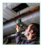
Extech Borescope features a 2.4" color monitor with video output for viewing on any monitor and a waterproof 9mm camera with bright LED lights.
