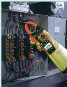
True RMS meter gives you accurate readings of non-sinusoidal waveforms.
