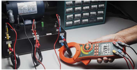
Connects to all three voltage phases simultaneously without having to move test leads from phase to phase.
