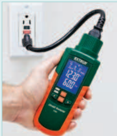
Tests 3-wire standard GFCI receptacles.
